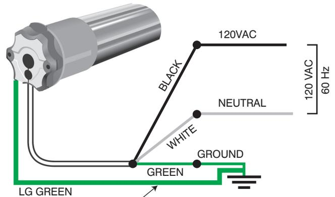
This extra ground wire is to ensure that the shutter is properly grounded to prevent electrical shock. Connect this wire to the same ground as the motor ground in the motor cable.
