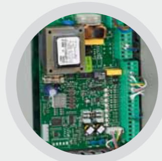
Integrated full feature control panel, easy to program through display and buttons, n°2 loop detectors control built in, full range of operating logics available (including logic PE). Control panel protected with metal housing and transparent cover to help service and maintenance.
